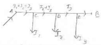
to the supply of feeding the distribution is connected to the supply of one end and loads are taken of differents along the length of the distribution.
