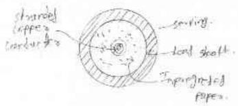
If consists of one circular core of linned orbranded copper insulated by Improgneted paper the insulation is surrounded by lead wheath. Finally serving is provided overTlead wheath to Protect the lead wheath from corrosion.
