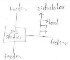
The radial system is employed only when power is generated at low nothinge and the substation is located at the centre of the load \* This is the simplex distribution cut and have lower initial cost
