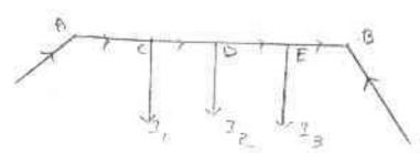
Cornected to the supply mains at both end & loads are tapped off all different points along the distributor.
